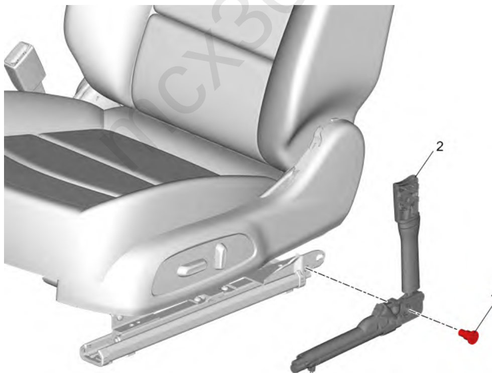
Fig. 26: Front Seat Belt Anchor Plate Tensioner Courtesy of GENERAL MOTORS COMPANY
